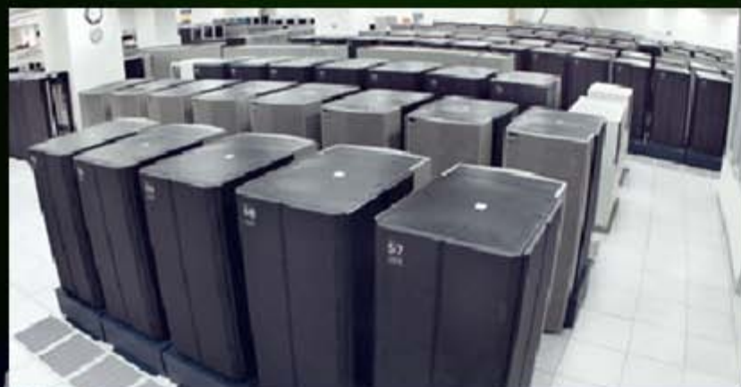
Seaborg: world ranking 14 (National Energy Research Scientific Computing Center at Lawrence Berkeley National Laboratory) IBM SP Power3 375 MHz 16 way / 6656 CPU / 9984 GFlops
